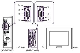
The arrangement of CANopen I/F and its peripheral equipment differs between the GP-3300/GP-3400 Series and the GP-3500/GP-3600 Series.
