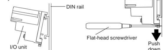
Be sure that the top and bottom faces of the unit are facing the correct direction and the unit is installed in a vertical position. Incorrect installation may prevent heat from dissipating.
