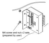
Fix the F9GT-HCNB on the panel face with M4 screws and nuts (prepared by user).
