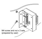
Fix the F9GT-HCNB on the panel face with M4 screws and nuts (prepared by user).
